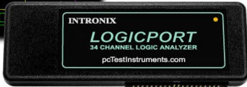
The LogicPort provides 34 channels sampled at 500MHz. This includes two state-clock inputs which function as normal sampled channels in timing-mode. The LogicPort is controlled and powered via your PC's USB 1.1 or 2.0 port for the ultimate in convenience and portability.
